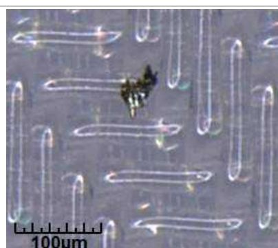
Fourth largest metallic particle 53 µm x 32 µm
